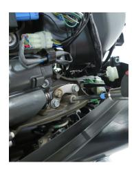
4. Insert the phillips screwdriver with the grip of the tool kit into the hole of the shift pivot.
