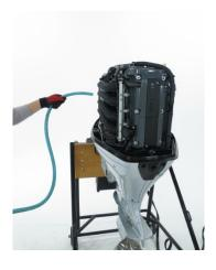
2. Rinse the outboard motor with fresh water to remove salt water, sand, mud, etc.
