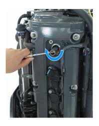
10. Carefully install the spark plugs by hand to avoid cross-threading. Tighten 1/8—1/4 turn after the spark plug seats.
