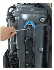
8. Remove the spark plug cover, all the ignition coil wire connectors, ignition coils and spark plugs.
