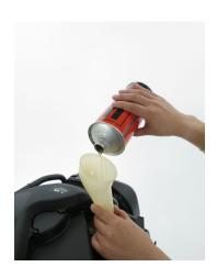
6. Refill to the upper level mark on the oil level dipstick with the recommended oil. Do not overfill. Too much engine oil may adversely affect the engine.
