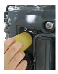
9. Pour a teaspoon of engine oil into all the spark plug holes to lubricate the inside of the cylinders.
