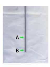
7. Check the oil level, insert the dipstick all the way to the engine then read the level. The oil level must be between the upper level (A) and lower level (B). If the oil level is correct, close the oil filler cap.
